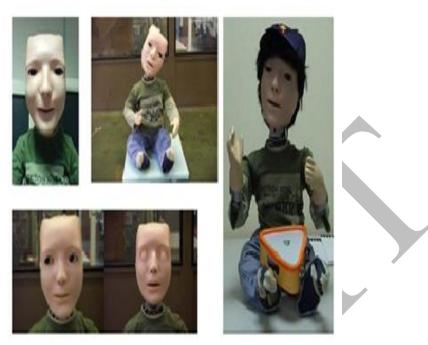
Figure 1. The minimally expressive humanoid robot KASPAR designed for social interactions
